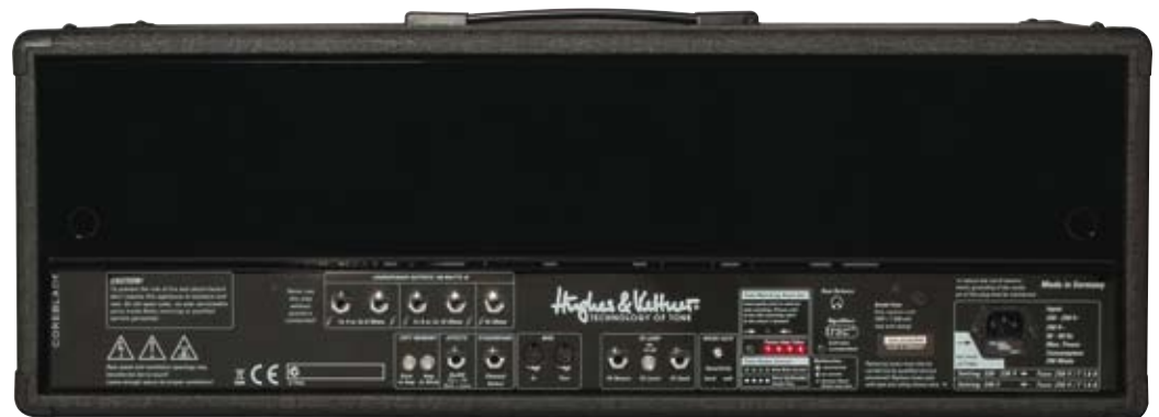
The rear panel, revealing the Coreblade's tube status monitoring features
